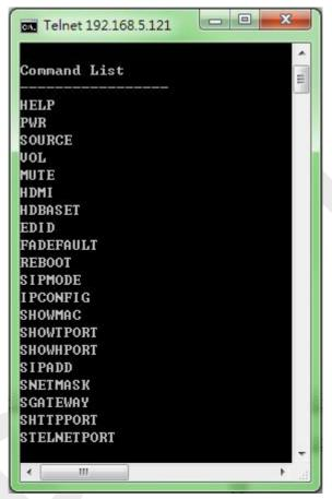
**Note:** Any commands will not be executed unless followed by a carriage return. Commands are case-insensitive. If the IP is changed then the IP Address required for Telnet access will also change accordingly.
