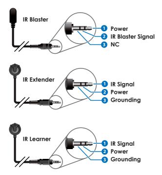
**Note:** Due to both IR Extender and IR Learner cables are with similar outlook, a part no. "CBL-IR10C3SA200A sticker has been placed to differentiate the difference on IR Learner.
