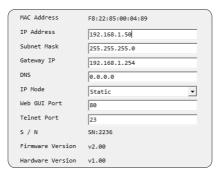
Then user may use the IP Address to find the control device through Telnet, WebGUI or even RS-232/Hyper Terminal tools.
