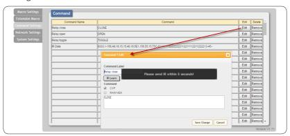
For IR command Learning, press IR Learn first then press the remote control in direct line-of-sight to the IR Reciever connected from the IRL port within 5 seconds. A command string will show in the bottom colum. Click on Save Changes to store the command.
